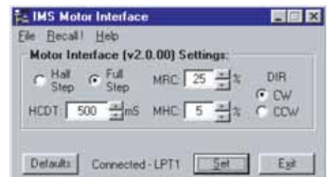
The IMS Motor Interface GUI simplifies MDrive configuring with a single screen interface.
